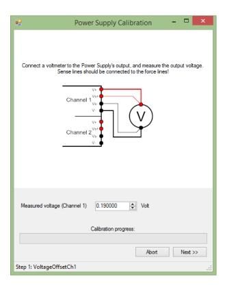
Filling in the DMM readings allows the calibration routine to verify both its programmed value and its readback value.
