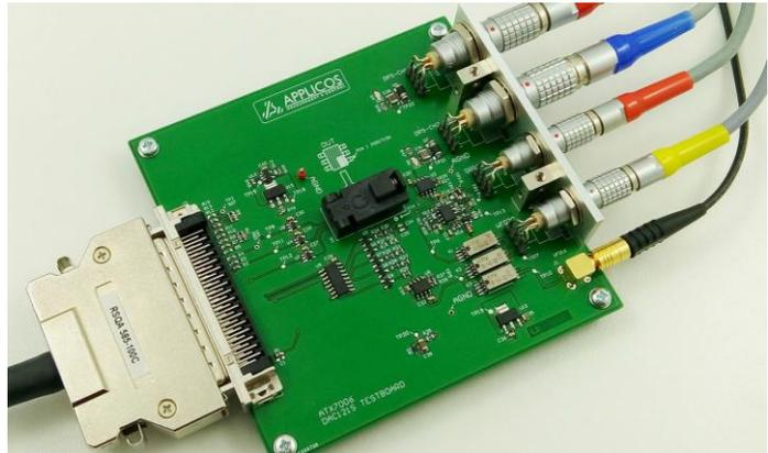
Test fixture with 4 analog signal connections
