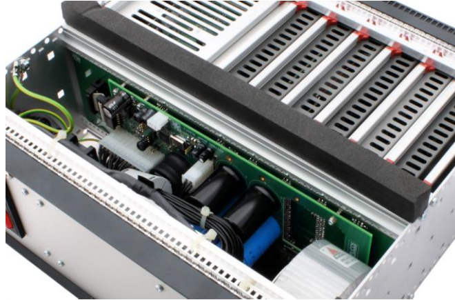
ATX-Express inside, screened modules, linear power supplies.
