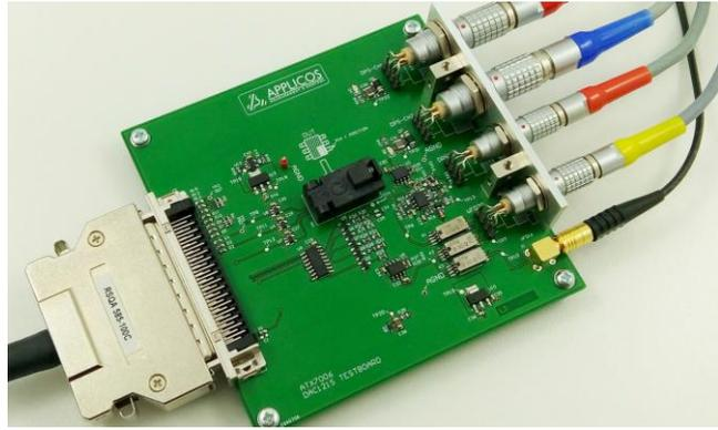
Test fixture with 5 analog signal connections.
