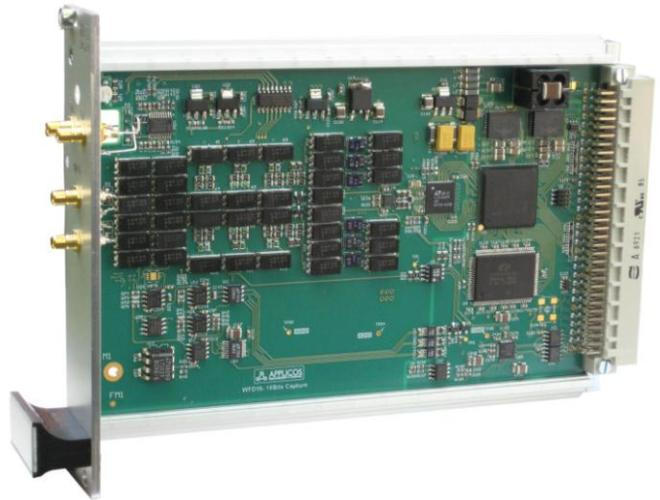
The WFD16 is a 16 bit Waveform Digitizer for high-speed / high resolution waveform capturing and analyzing. The fully differential signal path ensures an exceptional high signal quality. Despite this emphasis on signal quality the WFD16 also has a good DC accuracy.
